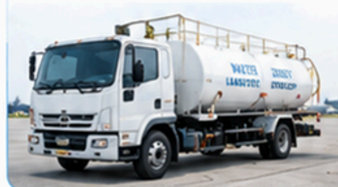
12 Water & Lavatory Service Vehicle
