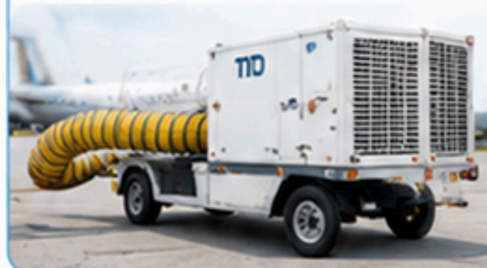
11 Ground Air Conditioning Unit
