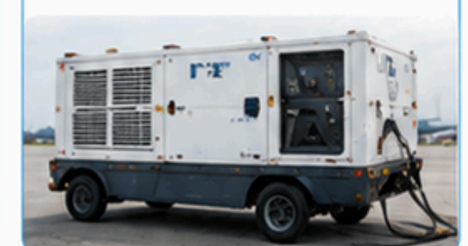
10 Ground Power Unit
